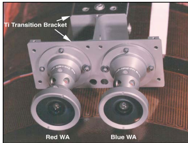
Figure 5. The MGS MOC wide angle camera heads prior to enclosure within the baffling structure. Compare with Figures 1 and 2 for scale ( figure5.jpg ).
