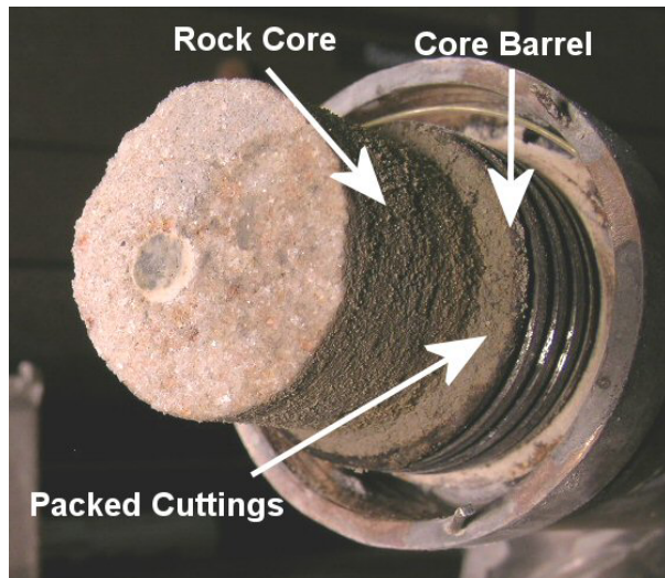
Figure 23. Cuttings packing around the rock core during the drilling process. ( figure23.jpg )
