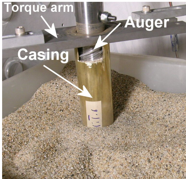
Figure 12. Experimental arrangement for observing choking phenomena. ( figure12.jpg )
