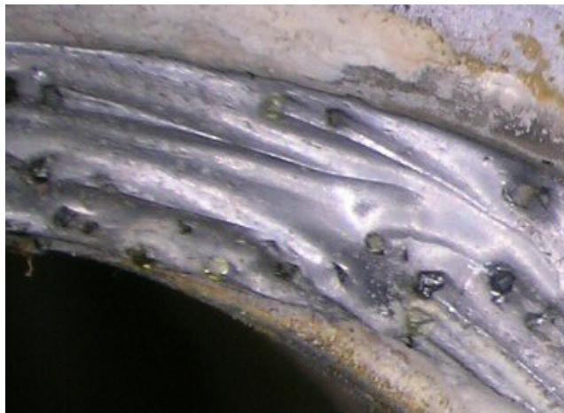
Figure 18. The wear of drill bit in frozen water saturated sandstone under Martian pressure. (a) The bit after being pulled out of the hole was clean. ( figure18a.jpg ) (b) Diamonds are replaced before they wear. ( figure18b.jpg )
