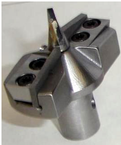
Figure 2a. The photo shows a bit with tungsten carbide (WC) cutters leaning 5^\circ forward or having a 5^\circ positive rake angle and held in place by a wedge and two set screws. The bit is a full faced bit with a centered WC spear point cutter (figure2a.jpg).
