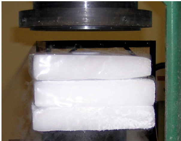
Figure 5. Test specimen inside the uniaxial test fixture. The top surface of the sample projects above the upper slab of dry ice ( figure5.jpg ).
