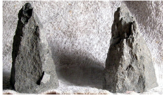
Figure 6. Conical fragments of basalt after unconfined compressive strength test ( figure6.jpg ).
