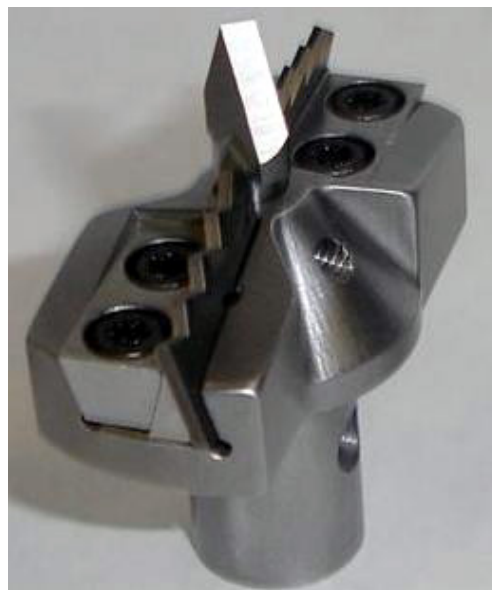
Figure 2b. The photo shows a bit with polycrystalline diamond compact (PDC) cutters leaning 15^\circ backwards or having a 15^\circ negative rake angle and held in place by two sets of wedges and set screws. The PDC cutter is made of a hard but brittle diamond layer (black and shiny layer) and a WC backing supporting the diamond layer. The WC backing is in direct contact with the wedge. In this particular design the PDC cutter has a serrated edge. The bit is a full faced bit with a centered WC spear point cutter (figure2b.jpg).
